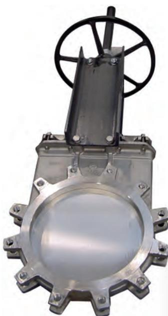
Unidirectional "Lug" knife gate valve (Bidirectional available), designed in accordance with standards MSS-SP-81 and TAPPI TIS405-8. Monobloc cast body with interior slides for optimum movement of the gate during operation. Provides high flow rates with low pressure drop.
