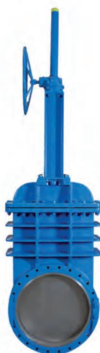
Unidirectional flanged gate valve (bidirectional option to order), designed for high pressure applications, with self-cleaning seal. Single piece die-cast body with screwed-down bonnet and wedges to guarantee the seal.
