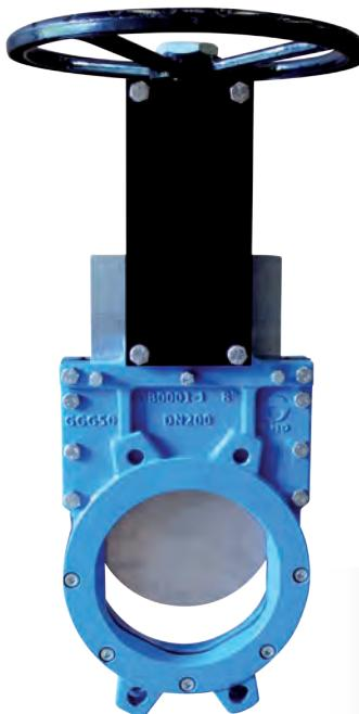
Bidirectional wafer-design knife gate valve. Two-piece cast body, joined by screws, with internal guides for smooth movement of through conduit during operation. Provides high flow rates with low pressure drop.
