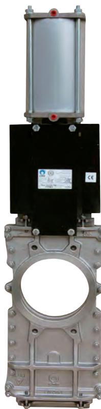
Bidirectional knife gate valve. Two-piece cast body, joined by screws, with internal guides for smooth movement of gate during operation. Provides high flow rates with low pressure drop.
